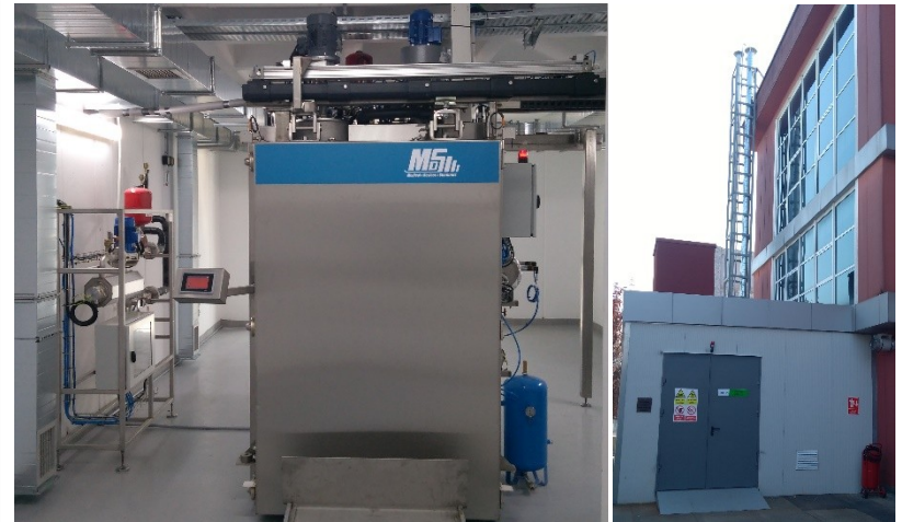
New ETO Sterilization System with Scrubber Unit for waste gas scavenging and recycling.
